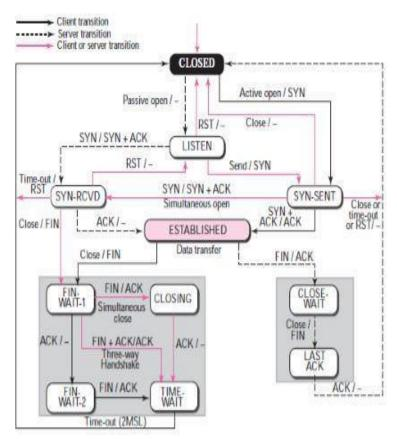
The figure shows the two FSMs used by the TCP client and server combined in one diagram. The ovals represent the states. The transition from one state to another is shown using directed lines.
